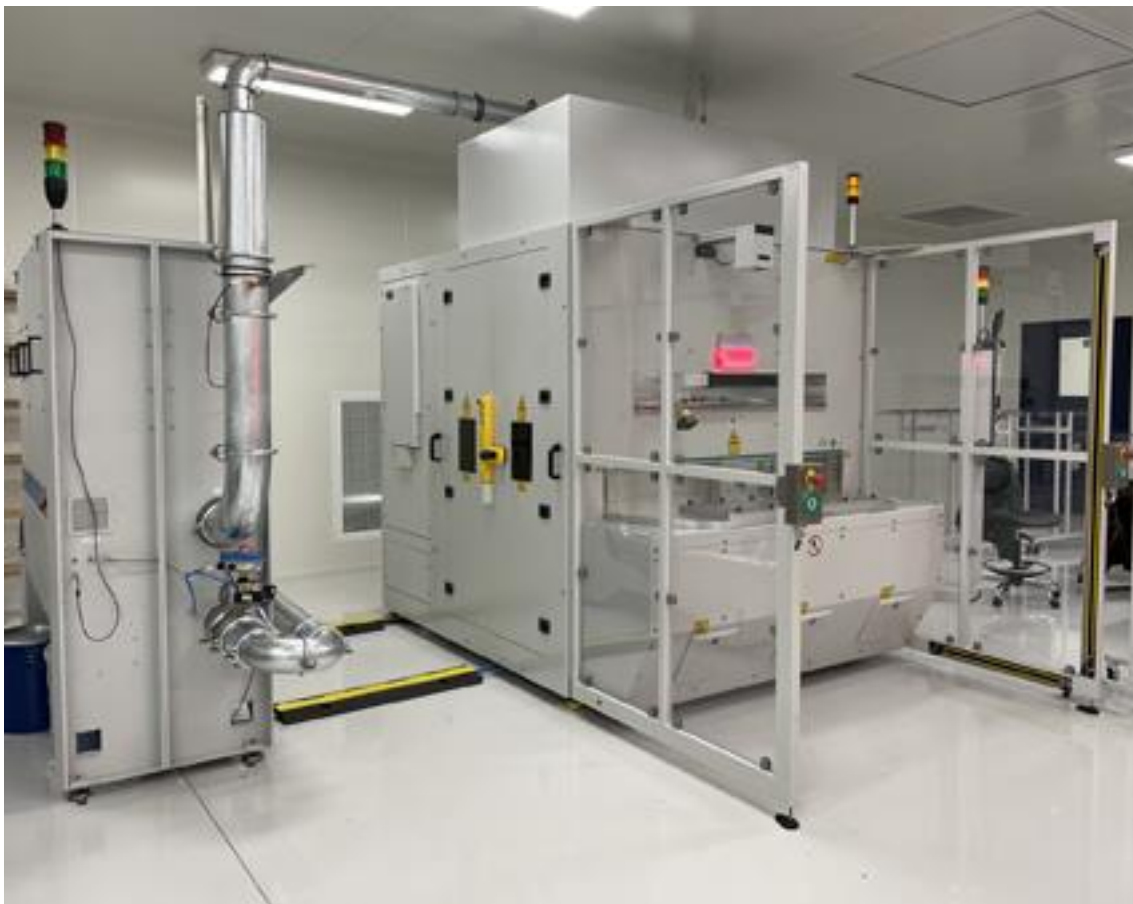
LAS 800 Ex fume extraction system (left) in use with a laser cleaning system from cleanLASER (©cleanLASER)
