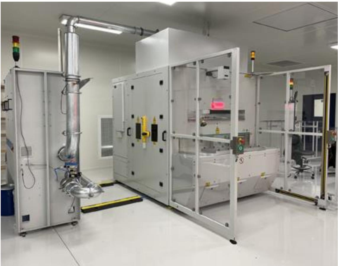
*Bild 4: Fume extractor LAS 800 Ex (left) utilized with a laser cleaning system*
