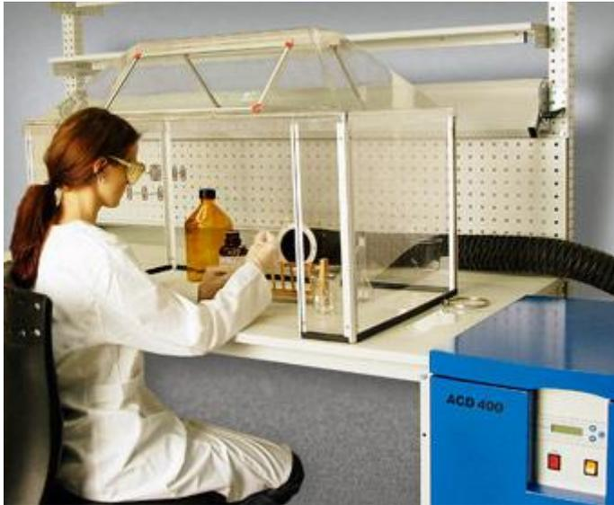
*Image 6: Half-open system as capturing element – connected to a fume extraction system via a hose*
