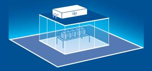
ULT develops special air drying solutions to be utilized in mini and macro environments. The production machine for battery cell production is completely enclosed or completely encapsulated and its air is dehumidified to the required level, depending on the process step between -20°C and -60°C dew point temperature. Additionally, the contaminated air is collected and filtered at the respective laser cutting and laser welding units.
