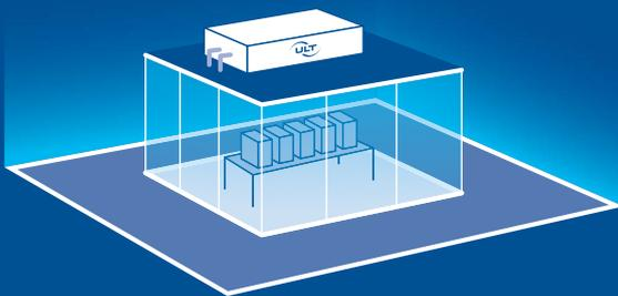
ULT develops special air drying solutions to be utilized in mini and macro environments. The production machine for battery cell production is completely enclosed or completely encapsulated and its air is dehumidified to the required level, depending on the process step between  $-20^{\circ}\text{C}$  and  $-60^{\circ}\text{C}$  dew point temperature. Additionally, the contaminated air is collected and filtered at the respective laser cutting and laser welding units.
