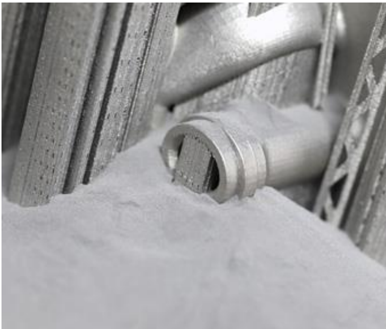
Image 2: Metal powder bed © Solukon
