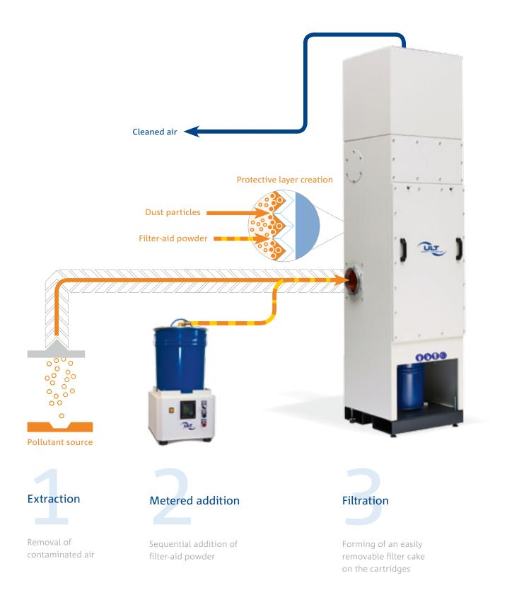
**Laser material processing** and many other production processes may cause extremely fine dusts. This emerges into a challenge for the filters in fume extraction systems – usually cartridge filter units.
